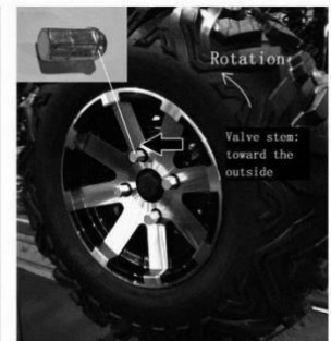
Rear Flange nuts:install with tapered side against wheel
