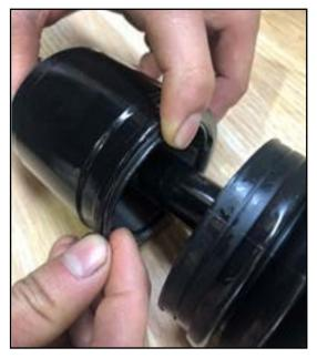
After taking out the retaining ring, you can directly pull out the intermediate shaft, pay attention not to drop the steel balls on the cage and the star sleeve, and clean the grease in the universal joint and the dust cover;
