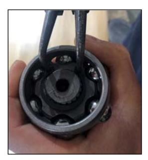
Use retaining ring pliers to remove the retaining ring of the star sleeve, after replacing the universal joint or dust cover, install the star sleeve in situ, and finally install the retaining ring;
