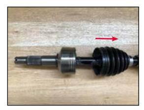
Remove the clamps at both ends of the dust cover, and pull the dust cover out for a certain distance along the direction of the middle axis;
