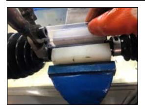
First install the small clamp, adjust the position of the dust cover to ensure that the dust cover is stuck in the groove of the intermediate shaft, and then use the clamp pliers to clamp the small clamp;
