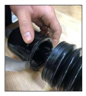
Use a sharper tool to take out the retaining ring in the universal joint;
